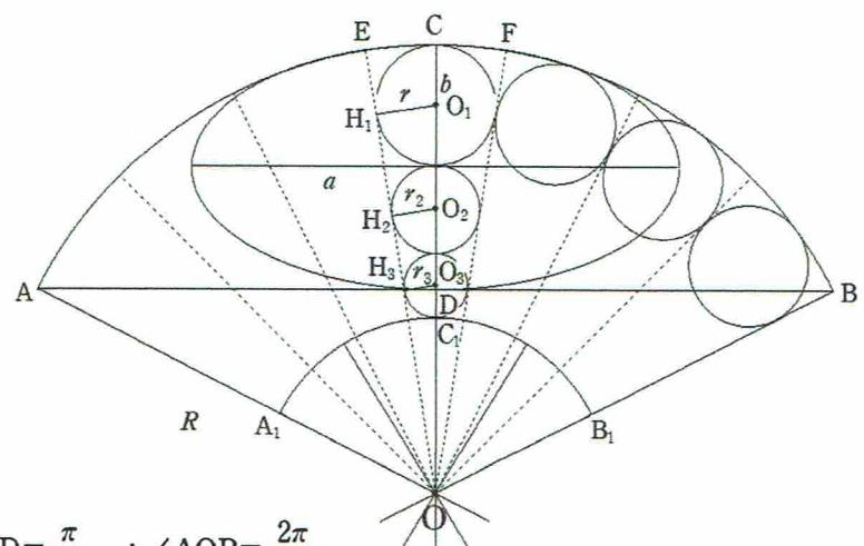
$$r_2 = \frac{1-\sin\theta}{1+\sin\theta} r, \quad r_3 = \frac{1-\sin\theta}{1+\sin\theta} r_2 = \left(\frac{1-\sin\theta}{1+\sin\theta}\right)^2 r,$$
